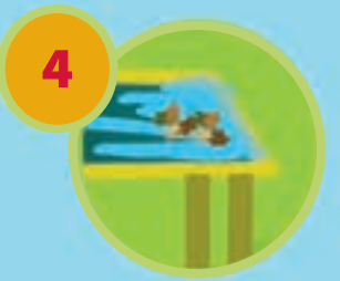
4 Flat roof with standing water.
