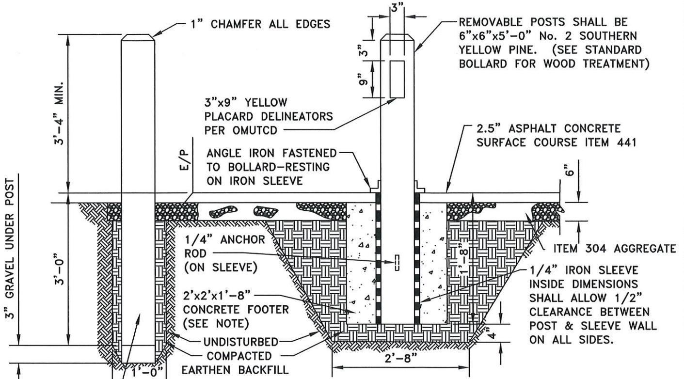
STANDARD BOLLARD - 6"x6"x6'-4" No. 2 SOUTHERN YELLOW PINE. ALL TIMBERS ARE TO BE TREATED WITH A.W.P.I. L.P. 22 (WOLMAN SALTS OR EQUAL) AND HAVE A RETENTION OF 40 P.S.F.
