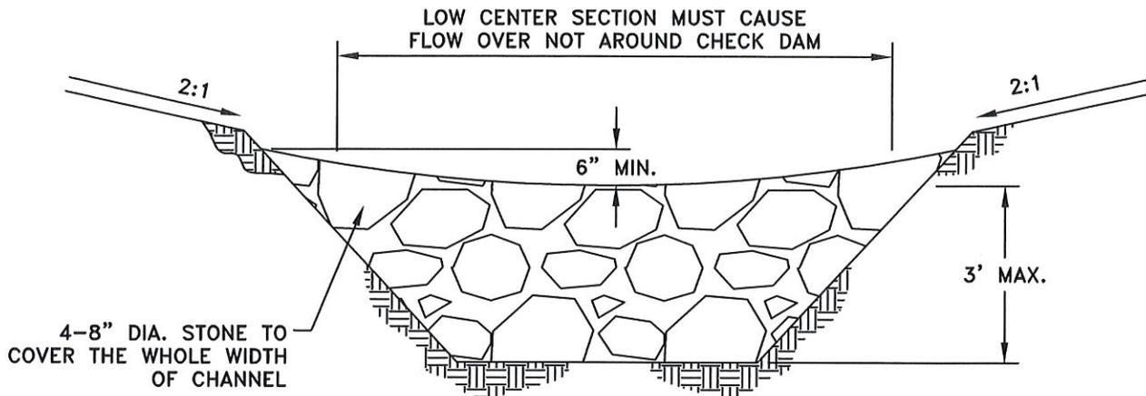
PROPER PLACEMENT OF A ROCK CHECK DAM IN A DRAINAGE WAY
