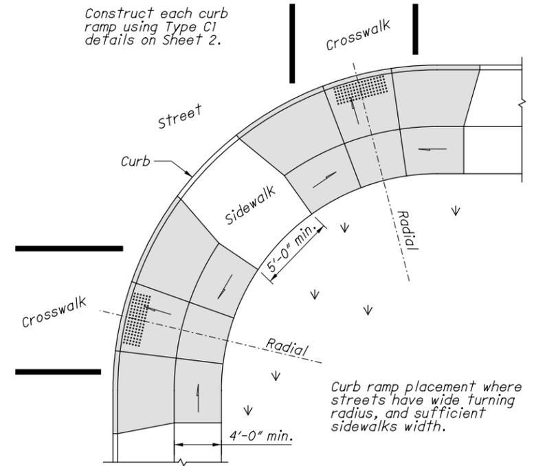
Construct each curb ramp using Type C1 details on Sheet 2.
