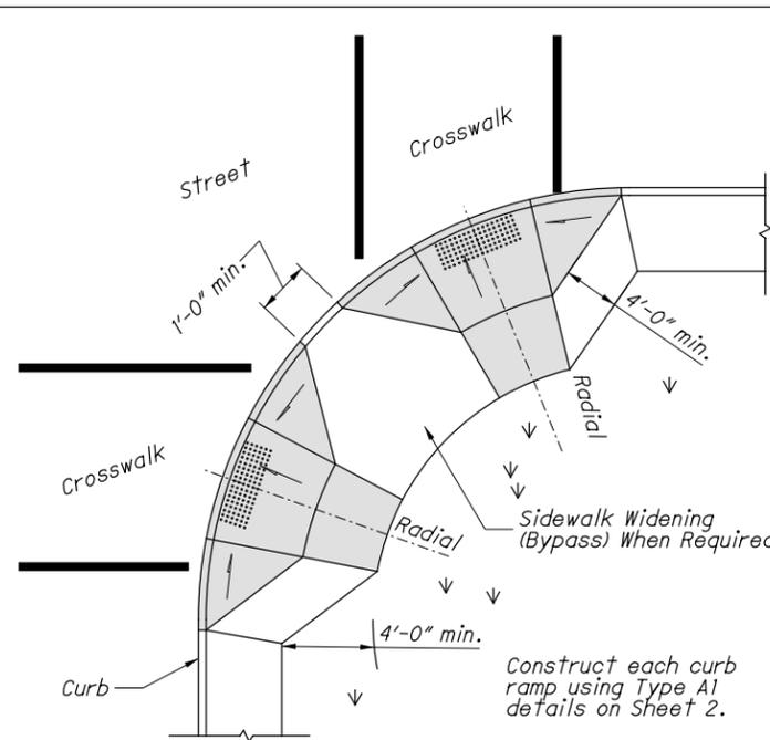
Construct each curb ramp using Type A1 details on Sheet 2.
