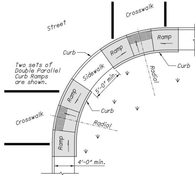
Two sets of Double Parallel Curb Ramps are shown.
