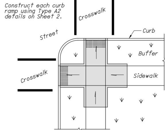
Construct each curb ramp using Type A2 details on Sheet 2.
