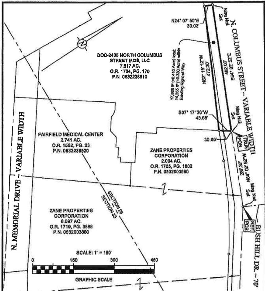
Basis of bearings is a northerly line of said 12.29 acre tract, also being a southerly right-of-way line of North Memorial Drive, being S 67° 08' 30" E, derived from a VRS observations referencing monuments, PID designation of D11868 and COR8 JD of OHHO, Ohio State Plane Coordinate System (South Zone - NAD 83, 2011 Adjustment), and all other bearings are based upon this meridian.
