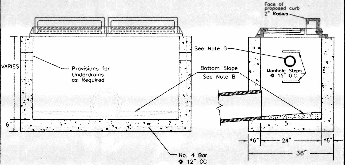
**NOTE A:** Cut-outs from pipes shall not be cut closer than 6 inches to an adjoining wall or top.
