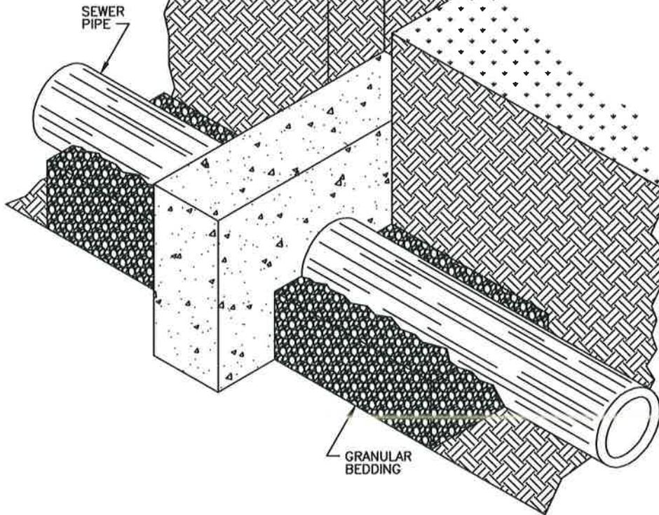
(\*) 2.5', OR A LENGTH SUCH THAT THE TOP OF THE TRENCH DAM IS 5' BELOW FINISHED GRADE, WHICHEVER IS GREATER.
