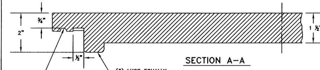
MACHINE GROOVE IN LID SEAT FOR OIL-RESISTANT T-GSKT NITRILE (60 DURO)
