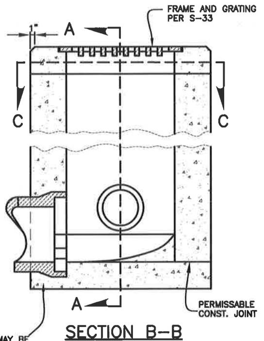
PRECAST BOTTOM SLAB MAY BE PLACED SEPARATELY. PLACE OUTLET PIPE WITH BOTTOM SLOPED TO DRAIN.
