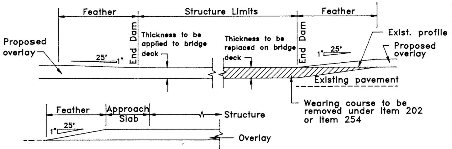
Detail assume non-settled approach slabs. Smoothing of the profile for settlement is required per plan grade or as directed by the Engineer.
