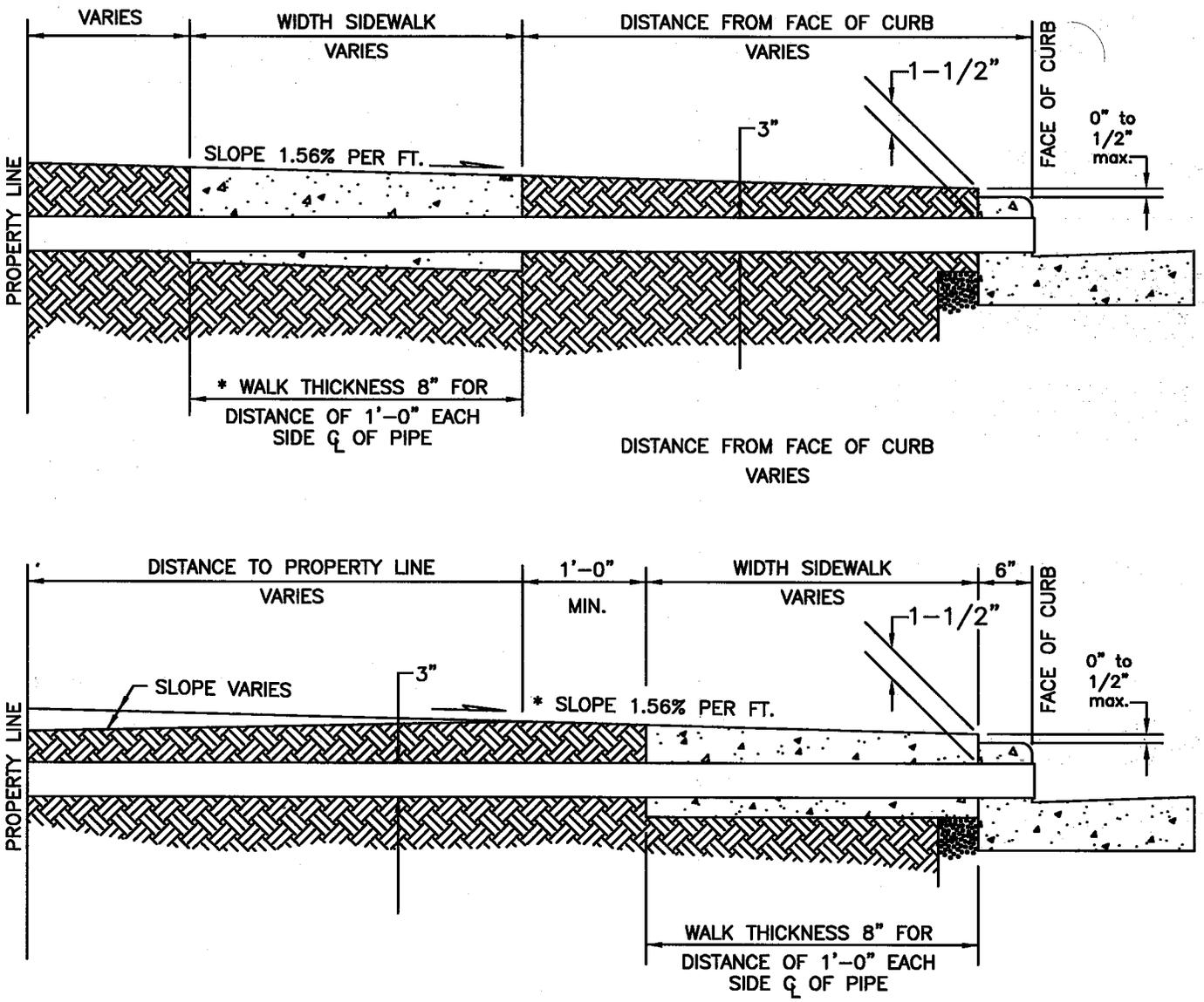
\* APPLICABLE ONLY WHERE THICKNESS OF CONCRETE OVER PIPE IS LESS THAN 4".
