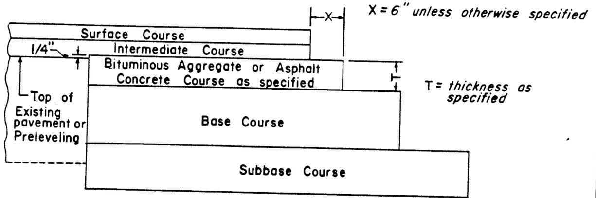
The Bituminous Aggregate in the upper part of the base widening shall finish approximately  $\frac{1}{4}$ " above the edge of the existing pavement where no preleveling is used. Where a preleveling (using intermediate course material) is specified it shall be placed prior to excavation of the widening trench and the upper course of the base widening shall finish approximately  $\frac{1}{4}$ " above the preleveling.
